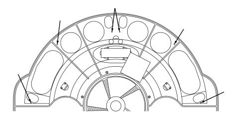
Lower the Ceiling assembly onto the top of the booth. Pass the wiring harnesses (not shown) through the holes directly above each harness so no wires get pinched beneath the Ceiling.
