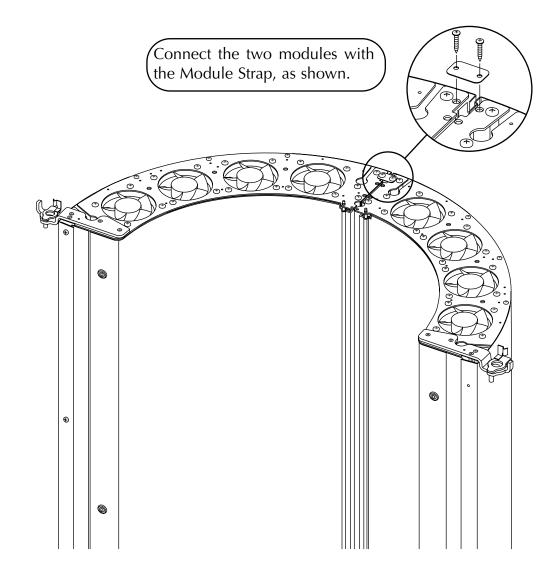
NOTE: Wiring deleted from illustration for clarity.
