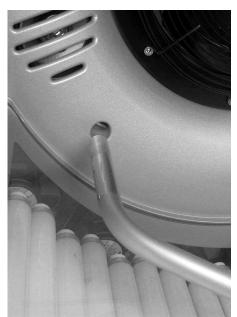
Slide the bottom of the handle into the lower handle bracket and insert a handle pin through it to lock the handle in place.
